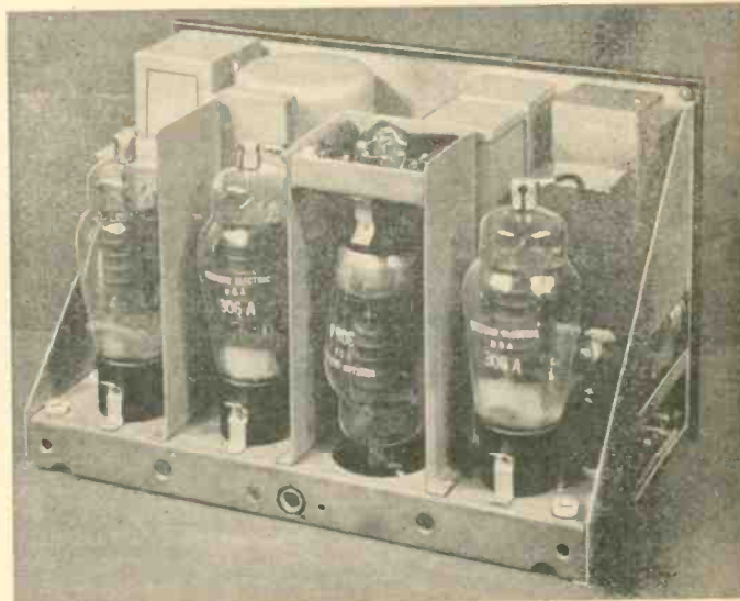
FIG. 1—Rear view of the chassis of the 18A Radio Transmitter. The harmonic generator tube is inverted to shorten the leads.
